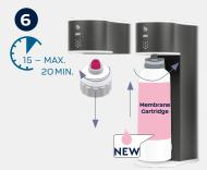
After the completion of the procedure unscrew the OsmoCare Adapter from the system and screw in a new Membrane cartridge.
